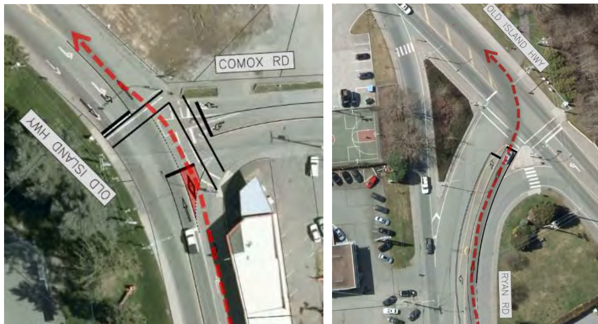
FIGURE 1. QUEUE JUMP LANE OPTIONS AT OLD ISLAND HIGHWAY / COMOX ROAD (LEFT) AND OLD ISLAND HIGHWAY / RYAN ROAD (RIGHT)
